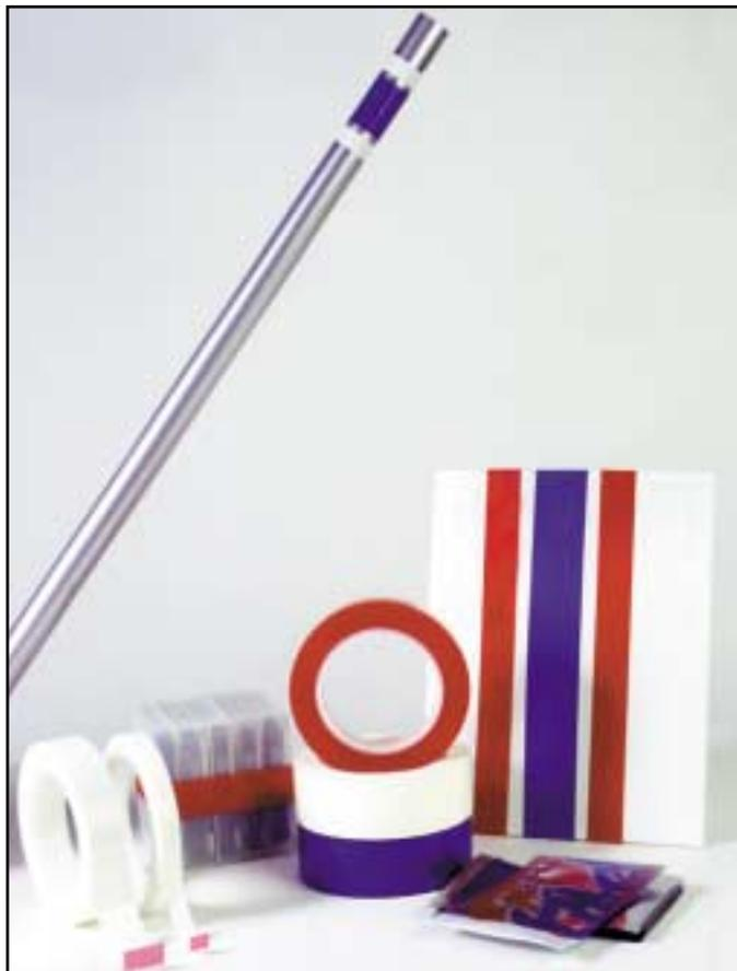
**Cleantack Cleanroom Tape™** is made of low density polyethylene film with pressure sensitive adhesive backing. This low particulate, contaminant free tape is wound on a clean plastic core and individually packaged in heat-sealed bags. Tape is produced and packaged in a class 100 cleanroom.
